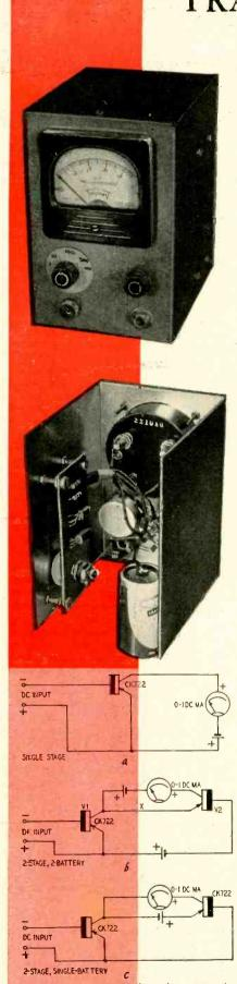
Fig. 2. To the simple two-stage transistor microammeter circuit of Fig. 1-c have been added the input multiplier resistors (R1 to R6) and the zero-setting meter circuit (R7 to R10). The zero-setting circuit is of the four-armbridge type common in v.t.v.m.'s.
